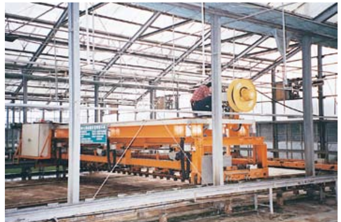
Moving Cart Motor Cable Reel
